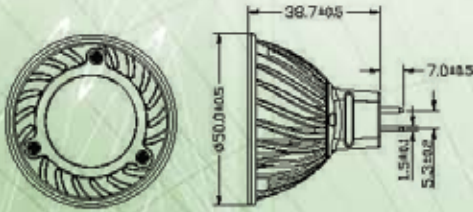
160 Lumens Turolux Vivid Solid State True Colour LED MR16 with CryoDrive (TM) Inside 3.5W Warm White or Daylight White
