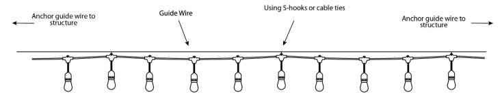
2. If a guide wire is not used, connect securely to structure at the beginning, middle and the end of EACH string light.
