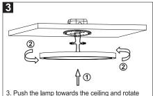
3. Push the lamp towards the ceiling and rotate the lamp to make the mounting plate and the lamp body fixed tightly.
