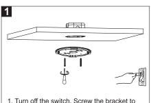
1. Turn off the switch. Screw the bracket to the junction box and ceiling.
