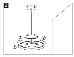
3. Push the lamp towards the hanging plate and rotate the plate to make the mounting plate and the lamp body fixed tightly.
