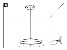
4. Turn on the switch to check if the lamp works normally.
