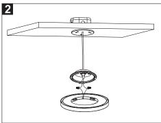
2. Connect the lamp body wires with power cord.
