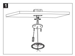
1. Turn off the switch. Use terminal caps to connect metal plate input line with power cord. Screw the metal plate in picture to the junction box and ceiling.
