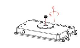
7.Put the input line in the embeddedbox passes through the waterproof pad and then passed through the lamp base.
