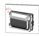
12.Lock the upper cover screws into the bottom shell with a cross screwdriver.
