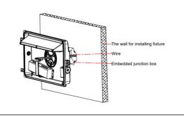
9. Connect the input wire and the dimming wire of the light, then put the connected wires into the embedded terminal box.
