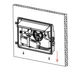
11.Insert the rotating shaft of the upper cover into the rotating shaft hole of the bottom shell.
