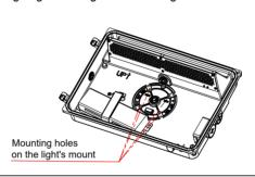
8. Usescrew to lock the lamp base on the embedded junction box. And ensure the balance of the horizontal column.
