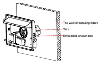
8. Use screw to lock the lamp base on the embedded junction box, and ensure the balance of the horizontal column.
