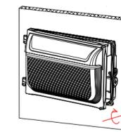
13. Fill the gap between the lamp and the wall with silicone sealant to prevent rainwater from entering the junction box.
