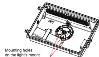
7. Put the input line in the embedded box passes through the waterproof pad and then passed through the lamp base.
