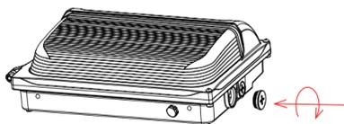
4. Use a screw driver to unscrew the lamp screws and remove the upper half of the fixture.
