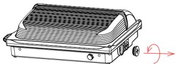
2. Adjust the power, color temperature, and light-sensing switches to the appropriate gear as needed. If the purchased lamps do not have color temperature optional or photocell sensor function, the color temperature optional or photocell sensor gear is empty.
