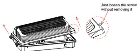
5. Unscrew the cover of the entry hole on the lamp base and remove the cover.
