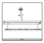
4. If wires are connected behind the fixture, carefully tuck the wires and wirenuts into the junction box before mounting the fixture. Align the fixture with the four (4) mounting screw heads so that the screw heads pass through the center part of the keyhole slots, slide the fixture to either side so that the screw heads are supporting the narrow slots of the keyhole profile.
