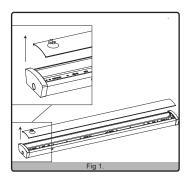
Remove the diffuser lens by using the supplied suction cup to lift up one end of the lens from the supporting channels. Once partially lifted up, the rest of the lens can be peeled back and completely released from the fixture body.
