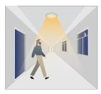
With insufficient daylight, the sensor turns light ON when motion gets detected.
