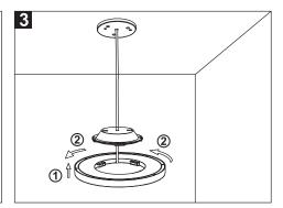
3. Push the lamp towards the hanging plate and rotate the plate to make the mounting plate and the lamp body fixed tightly.
