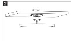
2. Connect the lamp body wires with power cord.
