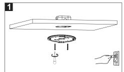
1. Turn off the switch. Screw the bracket to the junction box and ceiling.
