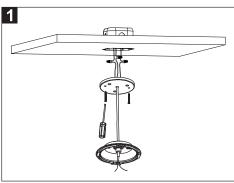
1. Turn off the switch. Use terminal caps to connect metal plate input line with power cord. Screw the metal plate in picture to the junction box and ceiling.
