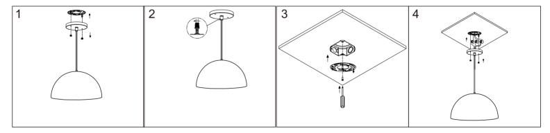
**Step 1:** Unscrew the two nuts, and then remove them from the lighting housing and mounting plate. Adjust the length of suspension wire by manually screwing the locking sleeve. The length range is 40-52inch.
