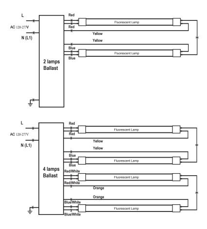
**Figure 2.** NOTE: For Double-ended, if the lampholders are non-shunted, the endcap close to the silver label should connect to the wires (yellow or orange). If not, some lamps will not function.
