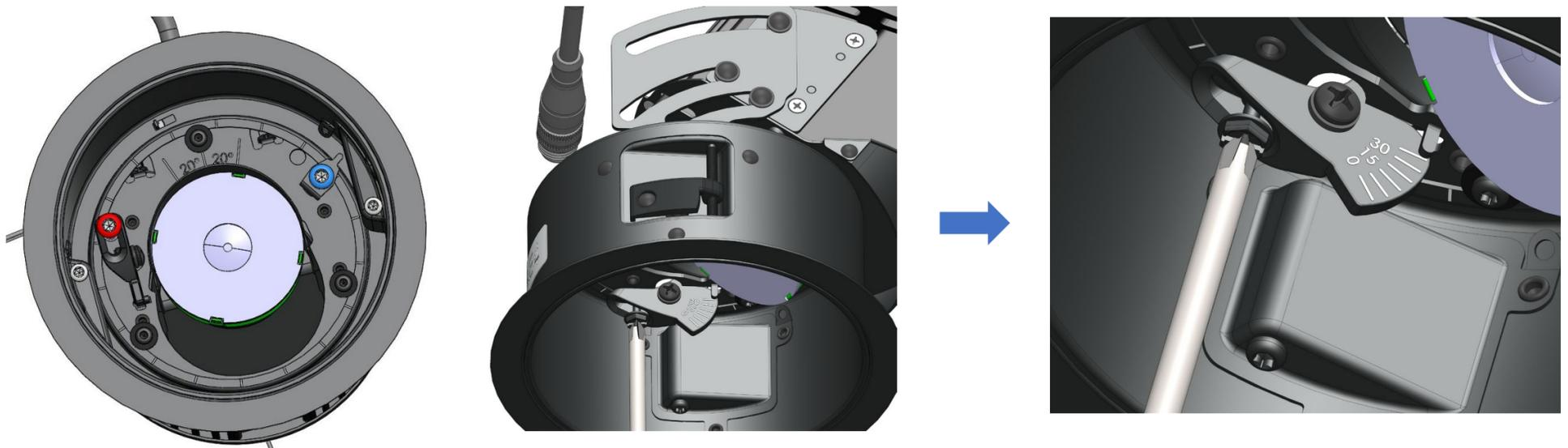
To adjust the tilting angle, tighten or loosen the **RED** screw with a T20 TORX screwdriver to the desired aiming point. For rotation loosen the **BLUE** and adjust to the desired position.
