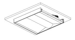
5. Place the last frame into the slots ,then slightly slide the last frame to the left , make sure it get locked tightly, join the last frame to the rested frames by fastening them together with appropriate fasteners .
