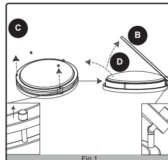
1. Loosen both nuts from the un-hinged studs as shown.
