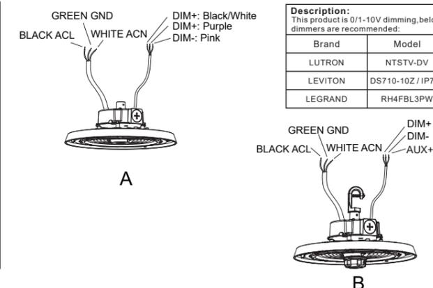
Please use the dimming+, dimming- (DC 10V) marking leads to connect to outside dimmer. The pink wire and black wire with shrinkable tubing shall not be damaged (no connection).
