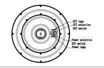
3.After finish the requires power and CCT adjustment, Tighten the M26 cap clockwise by slot type screwdriver.
