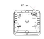
2.According to the tags,customer can select the corresponding power and CCT dip switch, dial to the required power(40w/60w/80w) and CCT(35K/40K/50K).
