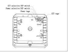
3.After finish the requires power and CCT adjustment, Tighten the M25 cap clockwise by slot type screwdriver.
