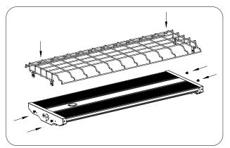
2.Insert the provided chips(4 pcs) onto the wire guard.
