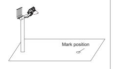
8. Turn on the laser device, then adjust the angle of stadium light, to make sure the laser can point at the marked place on the ground. Secure the bolt and screws by using the wrench and inner hexagon screwdriver, to complete the final installation.
