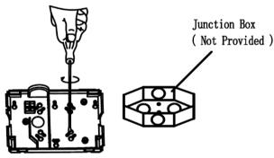
4.ELECTRICAL CONNECTIONS Make the proper supply wire connections.
