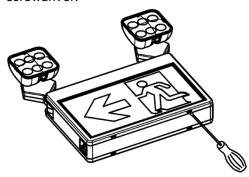
2. Knockout in back of mounting plate and push wires through the hole.
