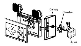
3. Reference 3 - 5 step in wall mounting above for side mounting.
