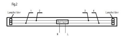
STEP 5: If the lampholder is not shunted, go to Step 6. If the lampholder is shunted, connect one lead from each lampholder to branch circuit as follows, "Leads 3 and 4" connected to L; "Leads 1 and 2" connected to N as shown in Fig. 2A. Cut as far away from the lampholders to allow for longer lengths of wire at both lampholders. Note: Ballast must be retained in place.
