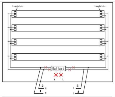
STEP 6: Connect any two of the leads to "L" and "N" as shown in Fig. 2B. Cut as far away from the lampholders to allow for longer lengths of wire at both lampholders. Note: Ballast must be retained in place.
